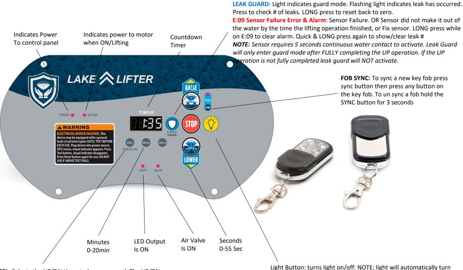
**SEL:** Selects the UP/DN timer to be programed. The UP/DN arrows will illuminate indicating which timer is ready for programming. HOLD the SEL button; when timer starts flashing use Mins & Secs buttons to set time.
