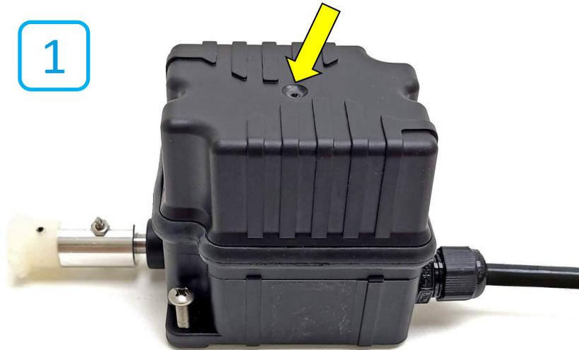
Open the rotary limit switch
