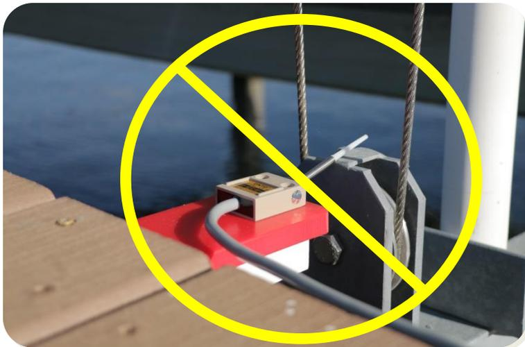
**UPDATE:** DO NOT install the limit switch where it will be tripped by the boat lift carriage. Continual non-stop movement of the carriage via wind will eventually wear out the limit switch. For longevity we recommend installing the limit switch where the cable is spooled.
