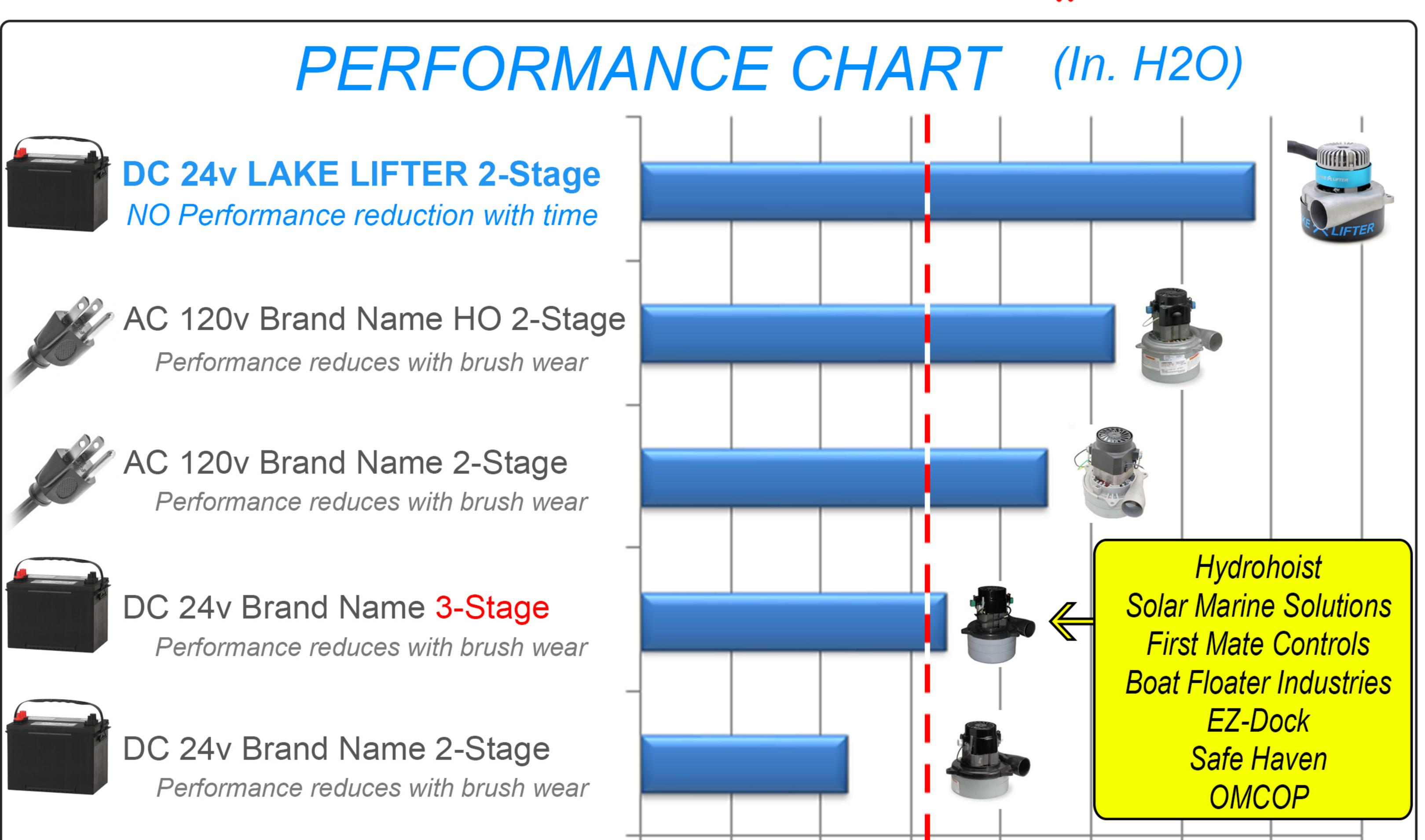
Minimum Required (In.H2O) For Air-Displacement Boat Lifts
