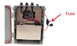
**NOTE:** The fuse is shipped disconnected. Insert fuse and close control box cabinet before operation.
