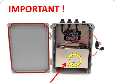
The battery should be mounted in the most upright position. If you mount the control box upside down remove the battery and flip it around so the battery will be up right after installing the control box.
