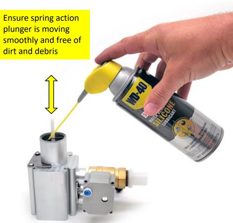
Use small amount of WD-40 or WD-40 Silicone lubricant on spring & inside body
