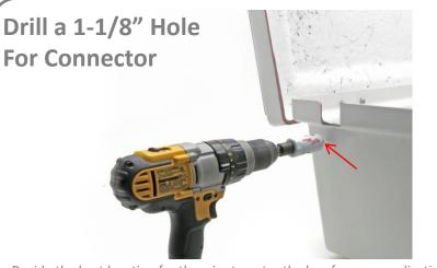
Decide the best location for the wire to enter the box for your application. The hole should be drilled just under the box lip as shown. For best results, use a 1-1/8" hole saw style drill bit to make a clean hole.
