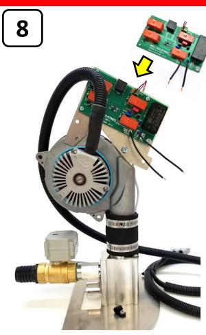
Re-attach the circuit board to the aluminum plate
