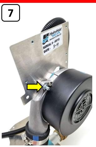
Tighten the nut on the back of the motor mount
