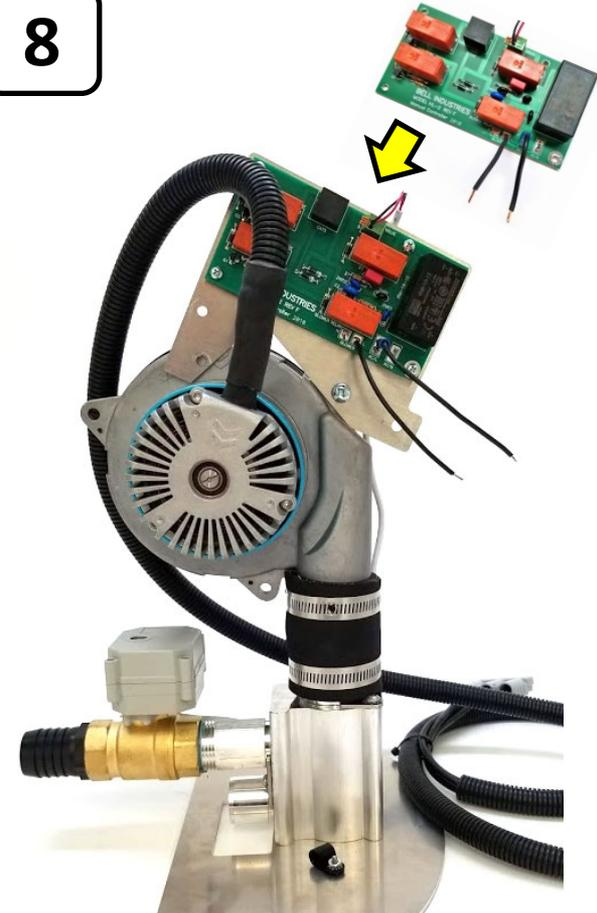
Re-attach the circuit board to the aluminum plate
