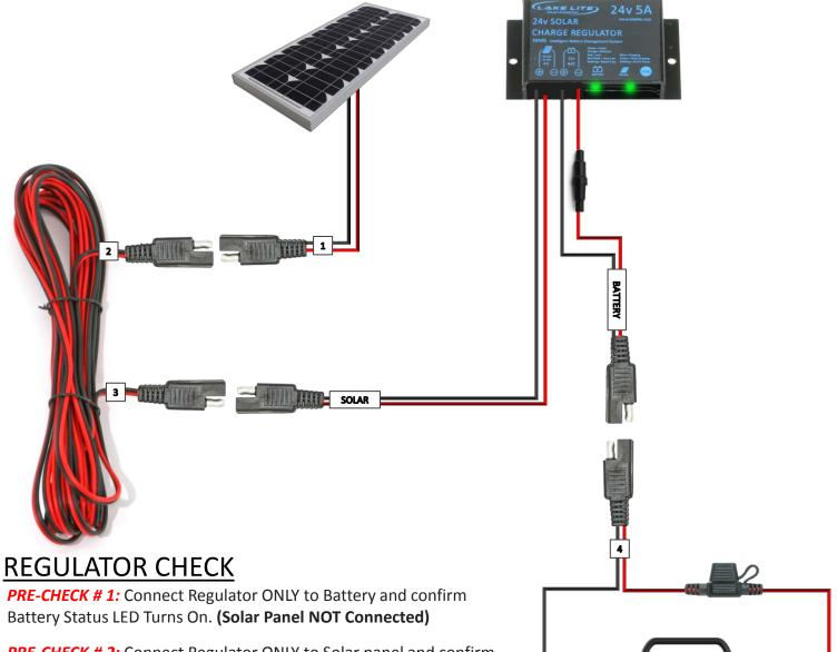
PRE-CHECK # 2: Connect Regulator ONLY to Solar panel and confirm Charging Status LED Turns On. (Battery is NOT yet connected)
