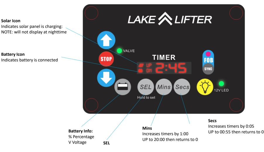
Short Press: Toggles between UP/DN timers Long Press: Enter program timer mode (flashing) Long Press Again = Set timer, or wait until timer stops flashing.
