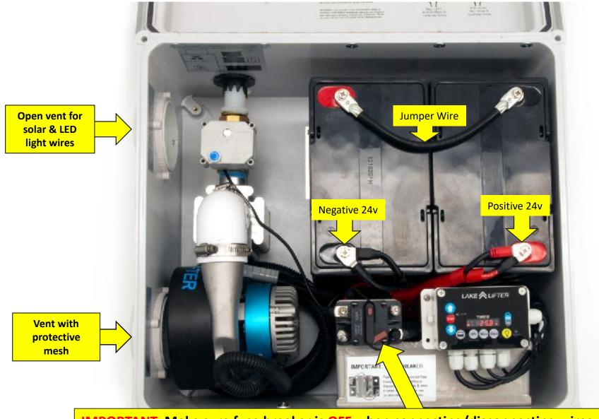
**IMPORTANT:** Make sure fuse breaker is **OFF** when connecting/disconnecting wires.
