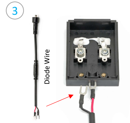
3 Insert diode wires, stagger the fork terminals for easy entry
