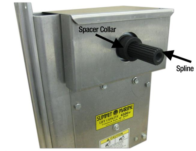
5. Install Spacer Collar and Spline.
