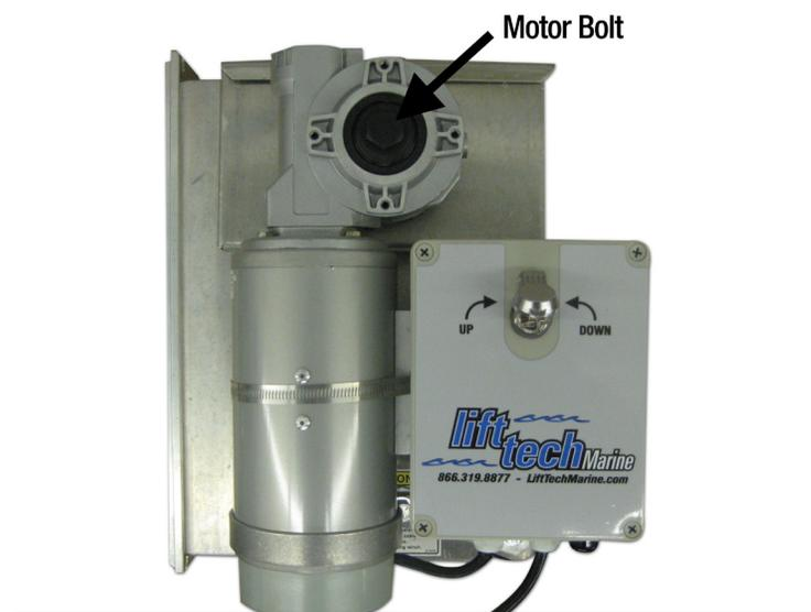
7. Install Motor Bolt and Washer. Tighten Motor Bolt to Approximately 70 Foot Pounds.
