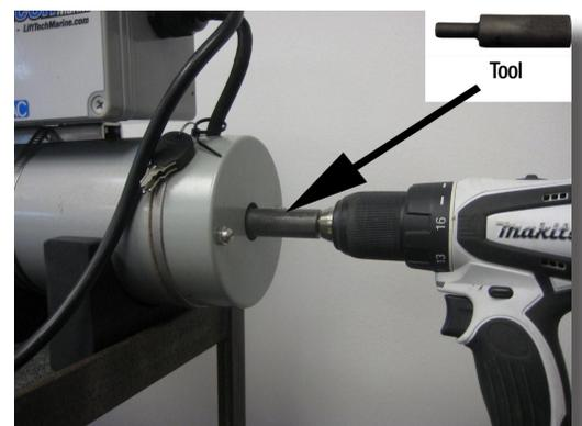
In Case of a Power Outage. This Tool May be Inserted Into a Drill to Raise or Lower Your Lift. First Remove Rubber Cap From Motor Shaft.
